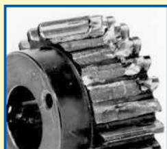
Example of the failure due to insufficient bending strength.
