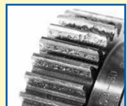
Example of the defacement due to insufficient surface durability.
