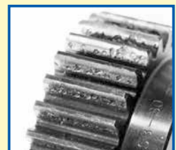
Example of the defacement due to insufficient surface durability.
