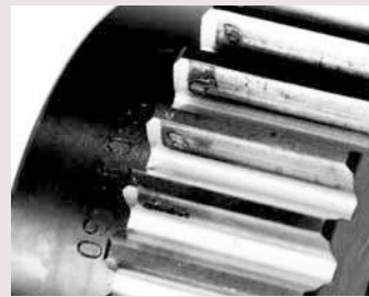
Poor tooth contact and pitting
