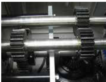
Full-automatic Forming Machine by Jey Machine Co. SSA and SS Spur Gears are used for stirring devices.
