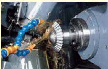
Gear cutting of Straight Bevel Gears
