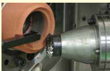
Gear cutting of Spiral Bevel Gears
